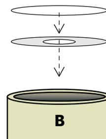
Apply glue to the ridge at end B, attach the paper circle with the hole in the center, and cover it with the last large transparent circle.
