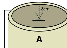
Roll the cardboard strip into a loose circle and insert it into the end of the tube marked A. Push the strip up against the tube ensuring the cardboard ring is snug and touches the can all the way around. The ends will overlap; mark the strip where the edges overlap and cut off the extra.
