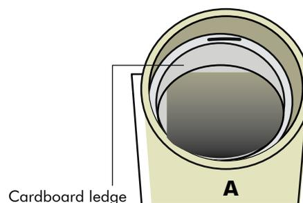
Take the small transparent circle, insert it into end A, and let it rest on the cardboard ring. Place colored transparent beads and plastic chips on the transparent circle.
