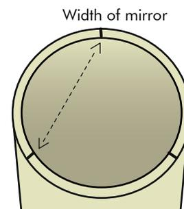
Insert a ruler inside end B until it touches the cardboard ring at the other end. Read this distance on the ruler. This distance will be the length of the mirror strips.
